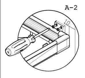
2- Fix the frame of shoes rack at a distance of 10 mm in front of the module from connection plastic with chip board screw. (A-2)
