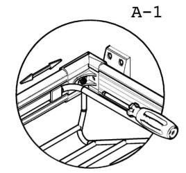
1- Loosen to screw on the corner plastic. Adjust according frame of shoes rack in width module. (A-1)
